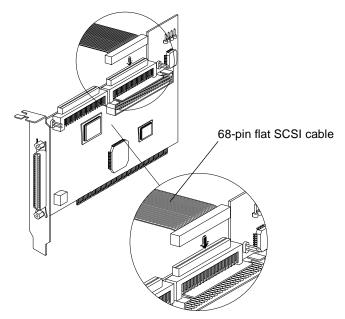
Figure 1-8. Connecting Ultra/Fast Wide SCSI Devices
